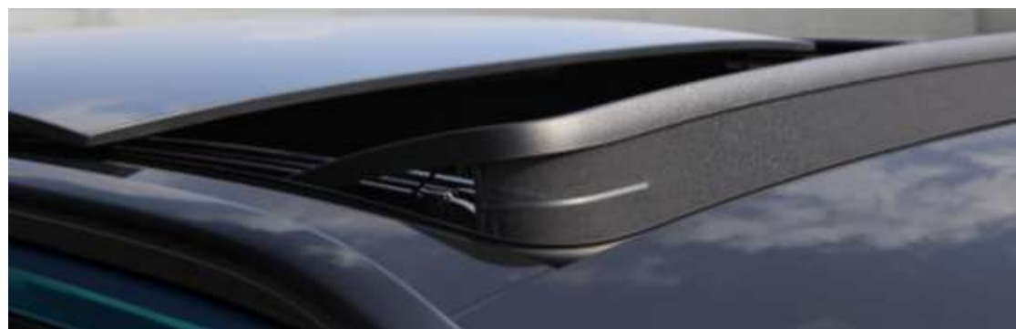
Spoiler Trapa electrica
