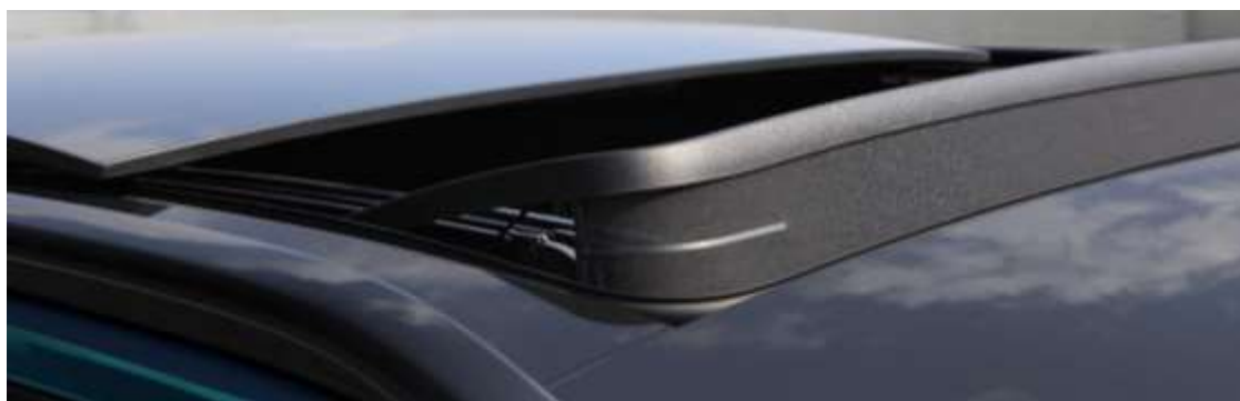
Spoiler Trapa electrica
